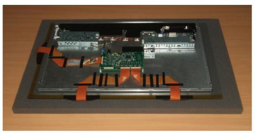
FIGURE 19 FINAL SOLUTION WITH ALL FLEXIBLE CABLES SECURED IN PLACE
