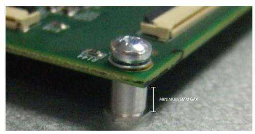
FIGURE 8 CONTROLLER SPACED 5MM ABOVE METAL WORK AND GROUNDED TO METAL CHASSIS VIA METAL STANDOFFS
