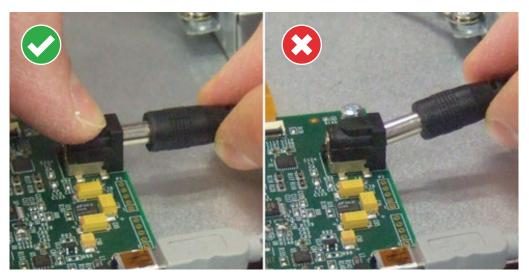
FIGURE 23 CORRECT AND INCORRECT POWER CABLE INSERTION INTO POWER SOCKET
