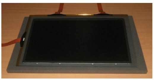
FIGURE 4 SENSOR MOUNTED ONTO LCD WITH GASKET
