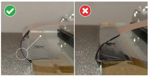
FIGURE 12 FLEXIBLE CABLE BENDING AT SENSOR EDGE
