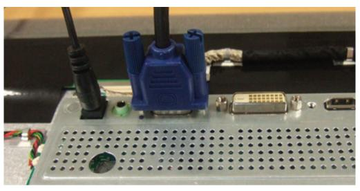
FIGURE 26 VIDEO AND POWER CONNECTIONS CONNECTED TO LCD
