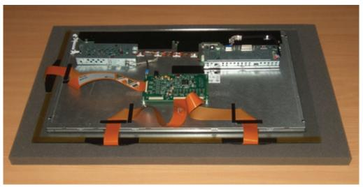
FIGURE 14 FLEXIBLE CABLES PLUGGED INTO THE CONTROLLER PCB
