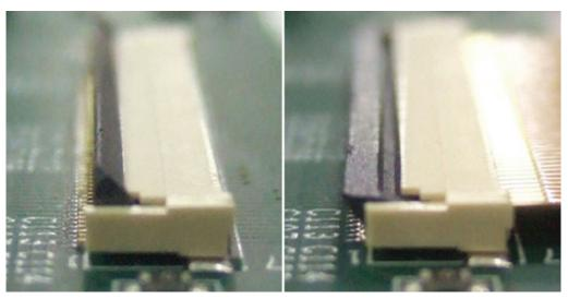
FIGURE 17 ZIF CONNECTOR LOCKING BAR IN UNLOCKED AND LOCKED POSITIONS
