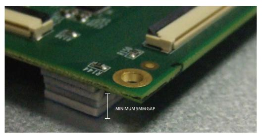
FIGURE 9 DOUBLE SIDED GASKET PADS MOUNTING OPTION
