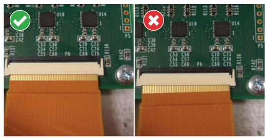
FIGURE 16 CORRECT AND INCORRECT FLEXIBLE CABLE INSERTION INTO ZIF SOCKET
