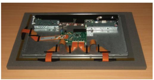
FIGURE 18 FURTHER BENDS AND TAPE APPLIED TO THE FLEXIBLE CABLES
