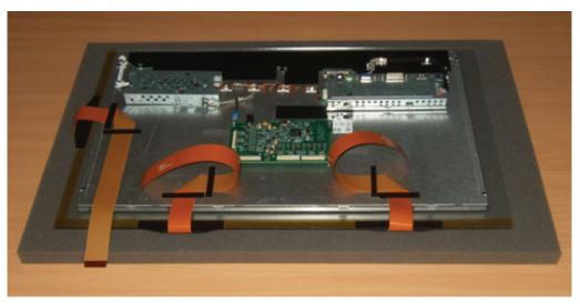
FIGURE 13 FLEXIBLE CABLES CAN BE CAREFULLY CREASED TO PRODUCE 90 DEGREE BENDS
