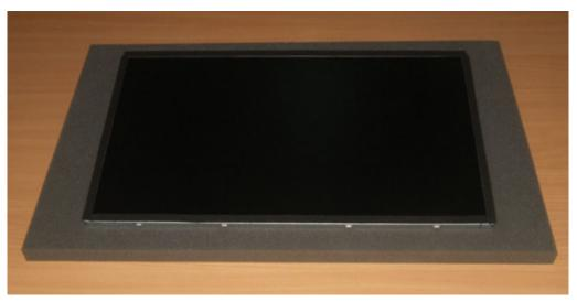
FIGURE 2 FOAM GASKET APPLIED TO LCD TO PROVIDE AIR GAP BETWEEN LCD AND SENSOR
