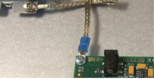
FIGURE 10 LOW IMPEDANCE GROUNDING CABLE
