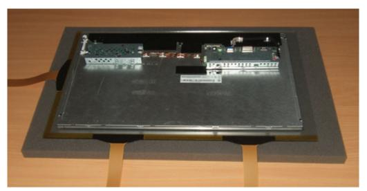
FIGURE 5 REAR OF LCD READY FOR CONTROLLER MOUNTING
