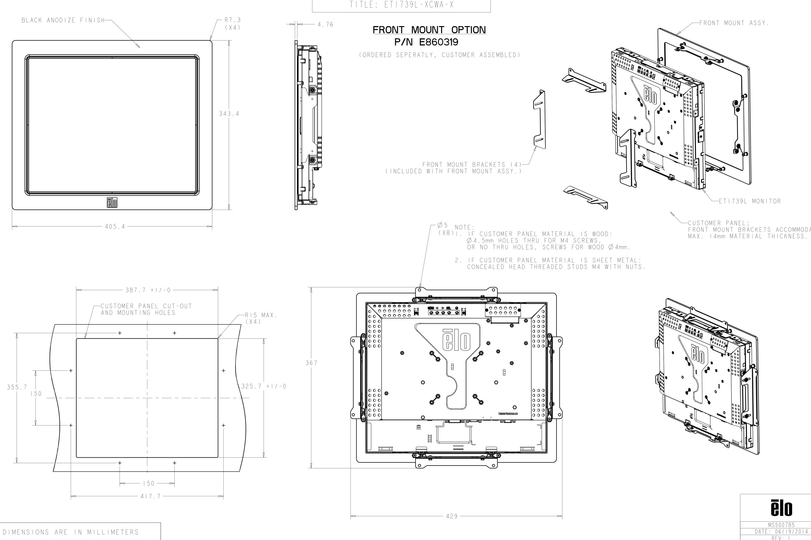
FRONT MOUNT BRACKETS ACCOMMODATE MAX. 14mm MATERIAL THICKNESS.
