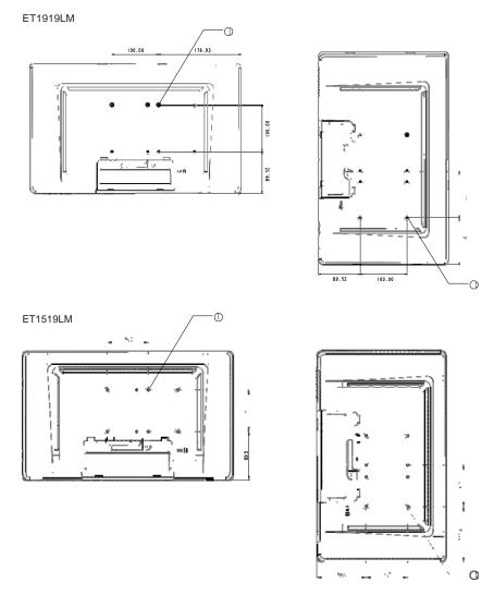
Figure 2-1: VESA mounting interface location, pedestal removed
